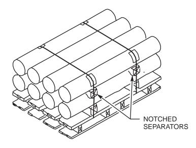
Figure 3. Items Secured to Prevent Rolling
