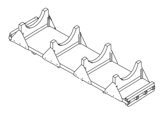
Figure 8. Cradle/Saddle Pallet for Cylindrical Items
