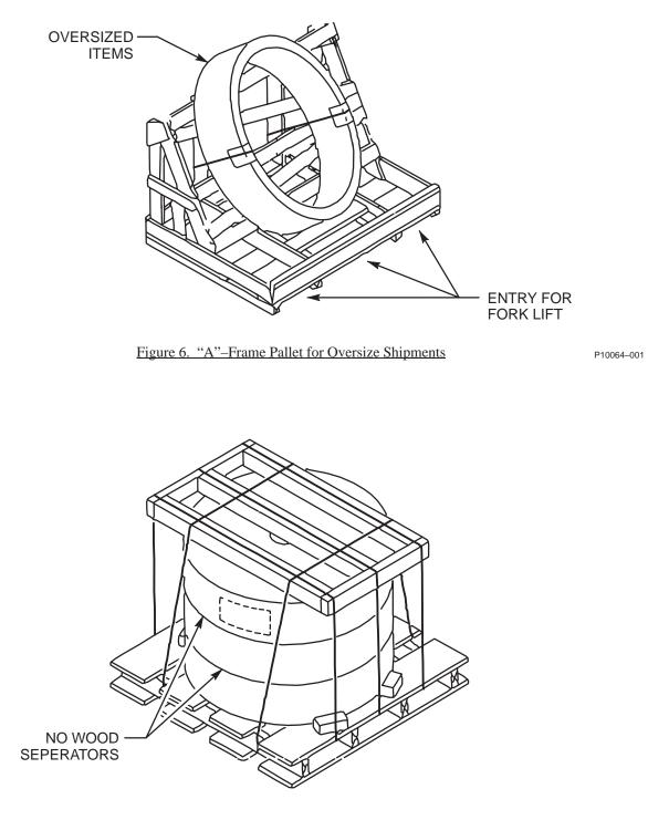
Figure 7. Items Stacked and Secured with Strapping
