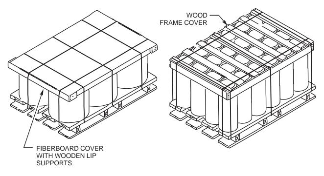
Figure 5. Items Secured (Bonded) with Cover
