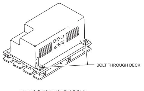
Figure 2. Item Secured with Bolts/Nuts
