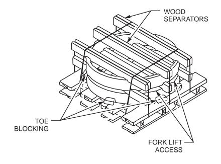
Figure 4. Items Stacked Permitting Forklift Access
